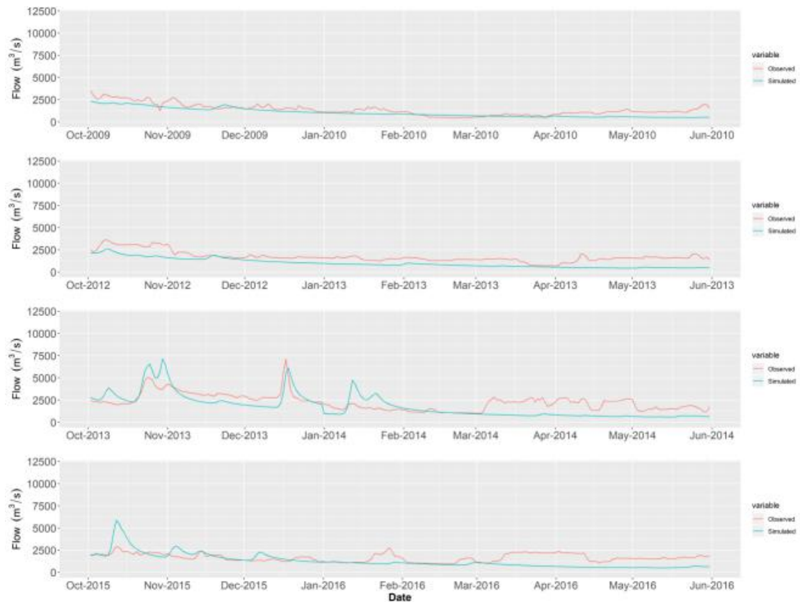
Figure 7.3-5 | Observed versus simulated flows at Chiang Saen for hydrological years 2009-2010, 2012-2013 and 2015-2016. Simulated flows represent flows under pre-dam conditions and observed flows represent flows under post-dam conditions. Differences between both curves were attributed to hydropower operations while congruence was attributed to climatic variability.
