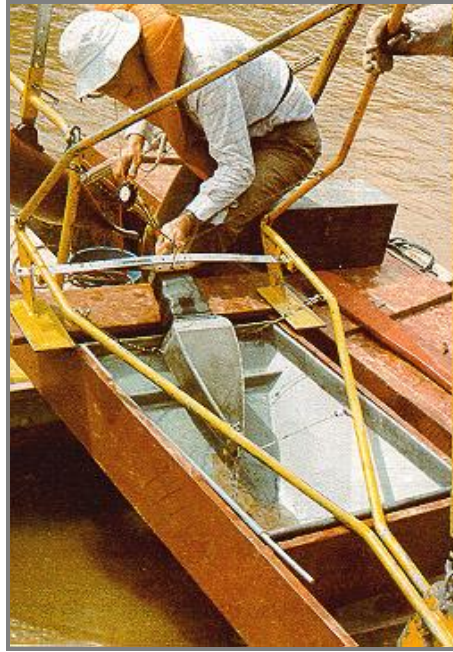
Figure 4.47 –Withdraw of sample in the entrainment discharge measurement using the sampler Arnhem. Coxim river, MS – IPH/UFRGS (02.03.1994).
