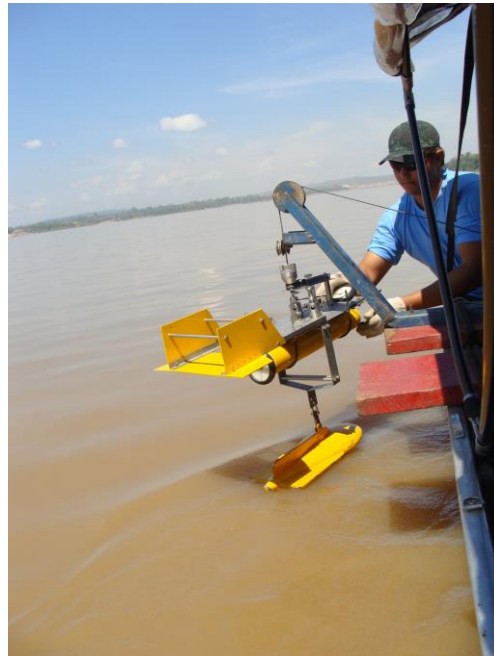
Figure 4.19 – Water sample collector for instantaneous of mixture water-sediment sample, used in Madeira River (Glenber equipment).
