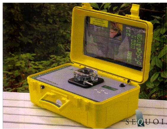
Figure 4.35 – Analyzer for granulometry and sediment concentration Lisst-Portable, of Sequoia (Carvalho, 2008)
