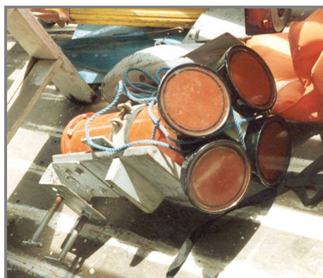
Figure 4.32 – ADCP (300 KHz) operating in Amazonia (Hibam Project).
