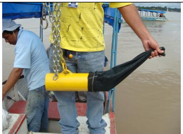
Figure 4.22 – A bed sampler for use in shallow waters
