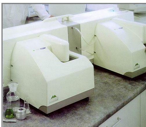
Figure 4.34 – Mastersizer that allows for granulometric analysis of the sediment, with few samples.
